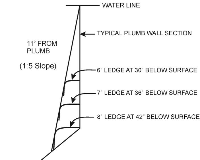
(9) **Underwater Seat Benches.** Underwater seat benches in pools, if provided, shall have a maximum horizontal seat bench depth of twenty inches below the waterline, be visually set apart by having the outer two inches of each seat lined with a slip-resistant tile in a contrasting
